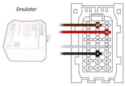
Brown (Emulator side) > Socket side, Pin20 Red (Emulator side) > Socket side, Pin16 White (Emulator side) > Socket side, Pin10 Black (Emulator side) > Socket side, Pin8
