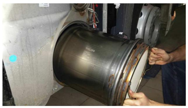
NOTE: Removing the DPF filters will be healthier. Otherwise, filters should be cleaned frequently by regeneration method.
